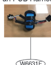
Inv PCB to Fan PCB Harness
